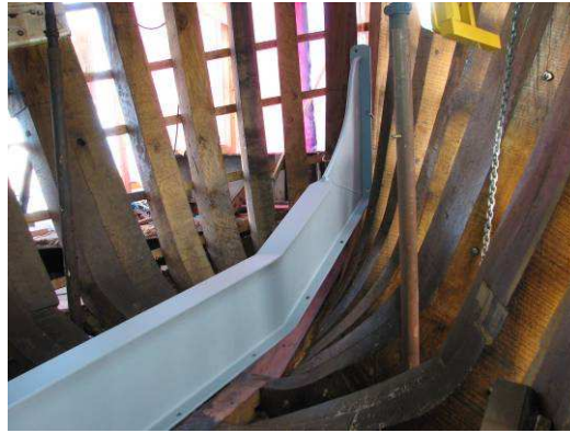
The refubished central keelson and complex frames at the bow
