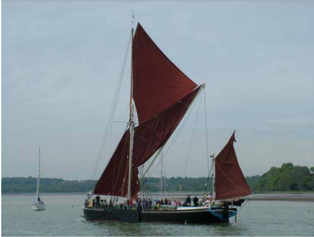
Victor with main half brailled up, sailing nicely and with iron tops'l
