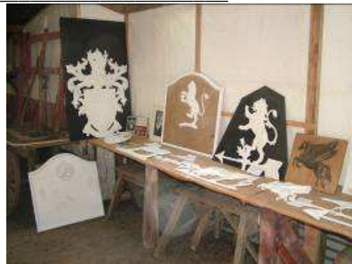
The early stages of creating the 'dies' for casting windvanes, signs, plaques, etc
