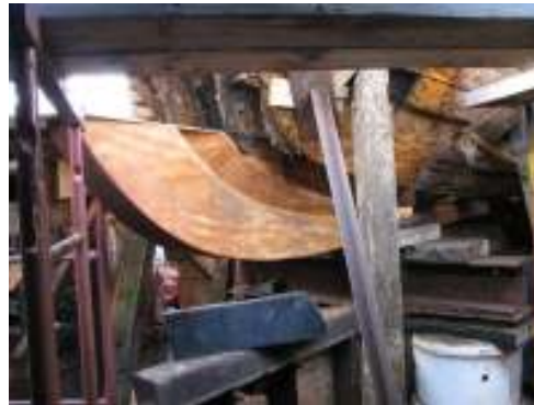
Fig 5 – November 06 – the worn forefoot replaced
