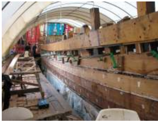
Fig 15 – December 07 – Hull planking nearing completion
