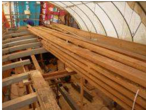
Deck planking prepared for installation
