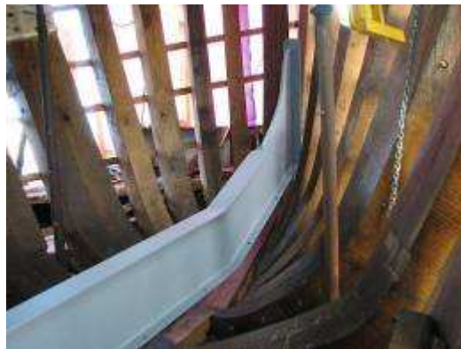
The refurbished central keelson and complex frames at the bow
